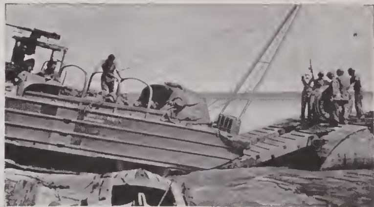
FIGURE 24. DUKW A-frame used to unload Signal Corps wire from causeway in southern France.
